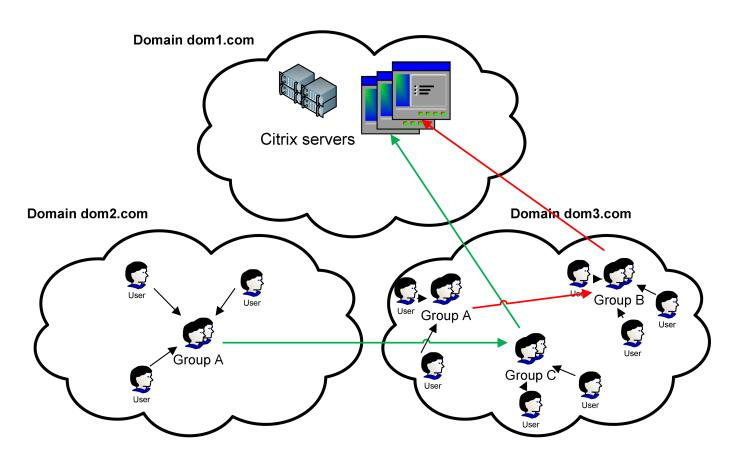
The above figure illustrates 3 domains (dom1.com, dom2.com and dom3.com) these domains are trusted. Dom1.com holds the Citrix farm servers and the three icons to the right of the server icon are the applications available to be used on the Citrix Farm. Group C from domain "dom3.com" got a reference to group A from domain "dom2.com". And group B from "dom3.com" got a reference to group A from the same domain.
